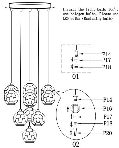
01. Unscrew the lamp holder ring (P18) counterclockwise, and then remove the iron tube (P17);
